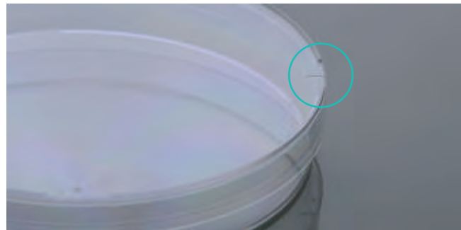
Vent points for Gas Exchange
