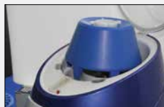
CoolTeenPrep™ Adapter 6 x 15 mL tubes Cat. No. 116002530
